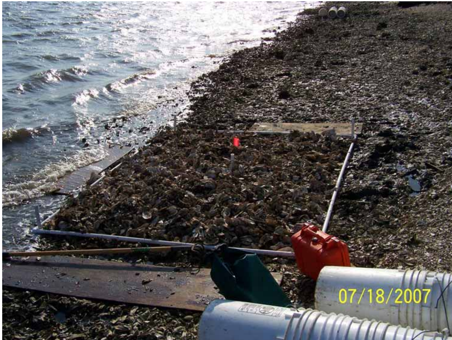
Block C, Rep. 3, Footprint 1. SC shell, 5 m 2 (used 25-6.5 gal buckets of shell)
