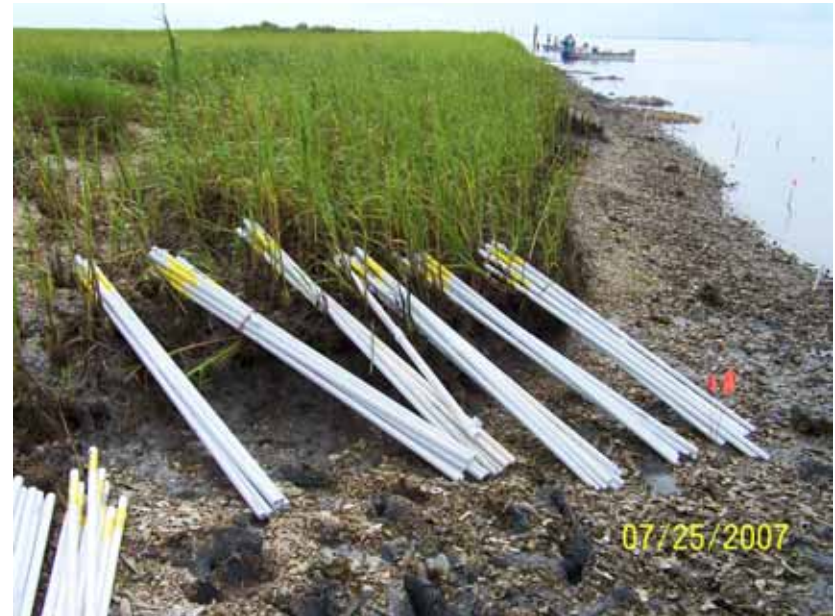
Raking out fossil oyster shell, R-292, setting up erosion poles/ GPS 'Trimbling' along the shoreline
