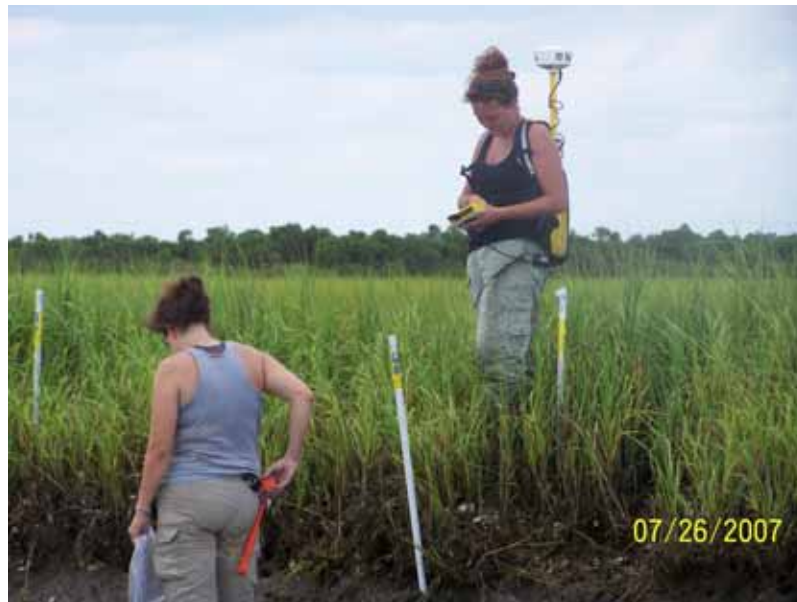
Raking out fossil oyster shell, R-292, setting up erosion poles/ GPS 'Trimbling' along the shoreline
