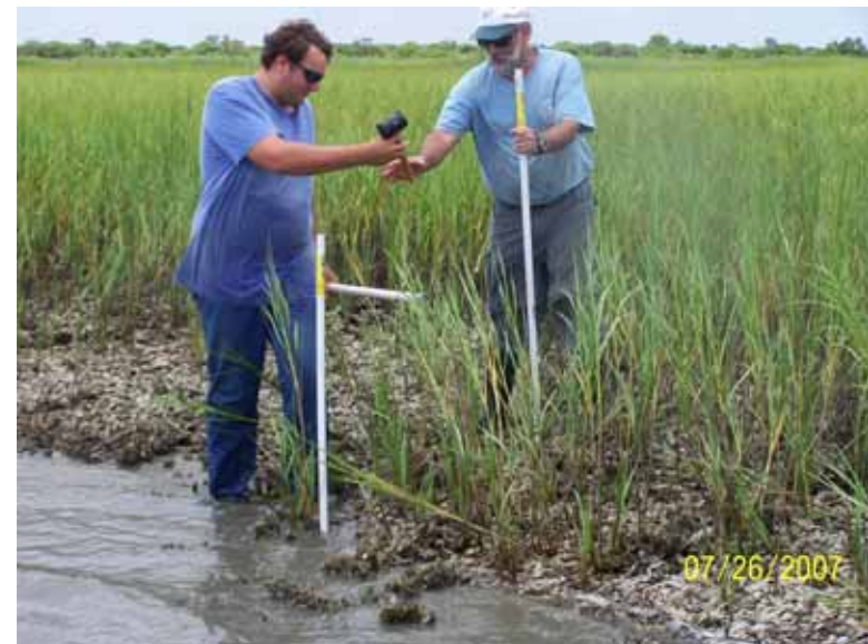
Raking out fossil oyster shell, R-292, setting up erosion poles/ GPS 'Trimbling' along the shoreline
