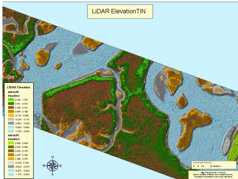
Figure 4.31 - LiDAR Elevation Last Returns TIN – BOB 4 Study Area
