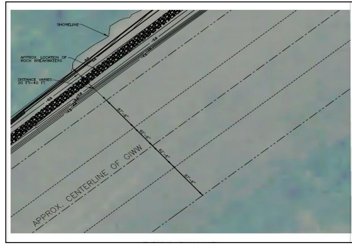
Figure 5. Typical Plan View of Breakwater Placement outside of GIWW ROW and Maintained Channel
