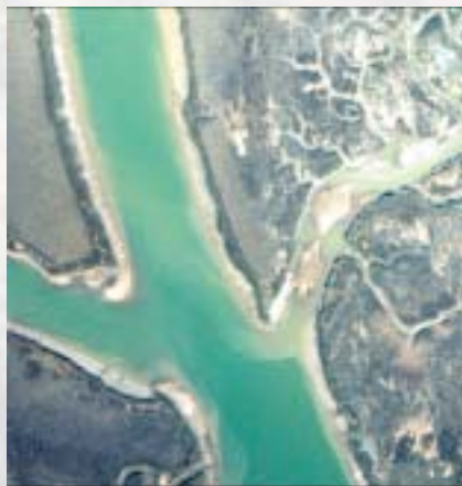
Conventional color aerial photography (Kodak 2448 film) flown at 1:5000 scale (2,500 feet altitude) over Hamlin Creek study area
