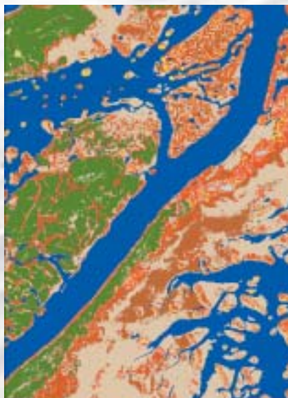
Upper Hamlin Creek study area classified data set. Produced by spectrally clustering GeoVantage 1/4 m imagery using NDVI and isodata algorithm
