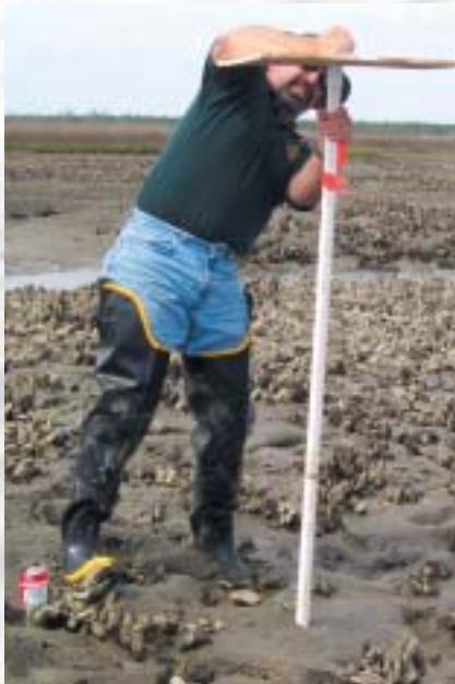
SCDNR staff setting up target over specific oyster strata to calibrate later overflight of GeoVantage imagery
