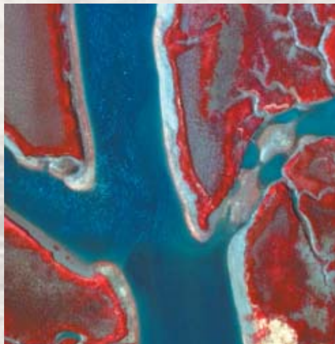
Geovantage false-color image (near-infrared, red, and green). Quarter-meter spatial resolution of Hamlin Creek study area.
