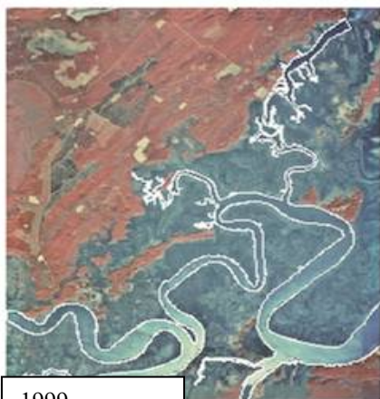
Figure 8: Shorelines were digitized from aerial imagery for the years 1965, 1972, 1979, 1999, 2005, and 2006. Imagery for 1965, 1972, 1979 and 1999 was scanned at 600 dpi.
