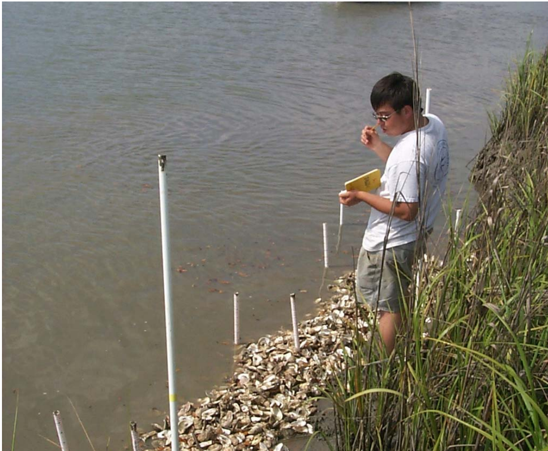
Figure 6. A small-scale experiments to assess the impact of boat wakes on newly planted Gulf shell, Inlet Creek experiments. Photo courtesy of Loren Cohen, Shellfish Research Section, Marine Resources Research Institute, South Carolina Department of Natural Resources, Charleston, SC.
