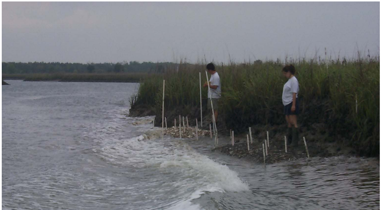
Figure 12. Small-scale experiments to assess the impact of boat wakes on newly planted Gulf shell, Inlet Creek experiments in April 2000. Photo courtesy of Loren Cohen, Shellfish Research Section, Marine Resources Research Institute, South Carolina Department of Natural Resources, Charleston, SC.
