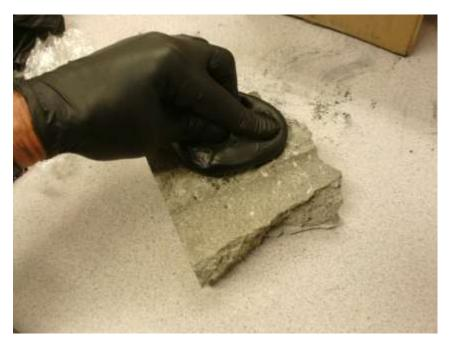
PRESS DOWN FIRMLY TO FORCE WATER OUT FROM BEHIND PATCH AND SPREAD OUT THE PATCH
