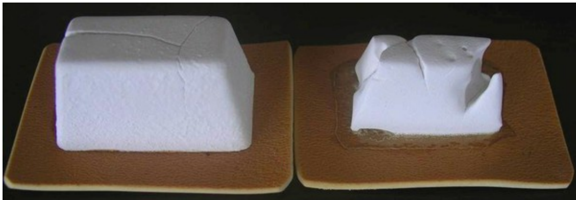
Figure 3. The control clod (left) will lose only a slight amount of weight while the experimental clod (right) will dissolve at a rate proportional to water motion.
