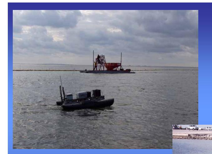
Unmanned Monitoring Vessel equipped with video and GPS data
