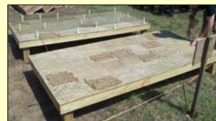
Control (right photo panel above) & plastic- (UV-opaque, OP-3 Acrylite®) covered platform (see left photo panel) with meshes in place
