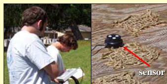
UV measurements being recorded using optical radiometer
