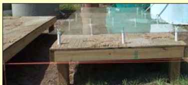
Control (right photo panel above) & plastic- (UV-opaque, OP-3 Acrylite®) covered platform (see left photo panel) with meshes in place
