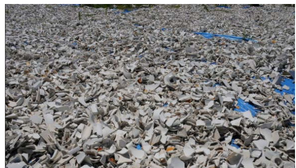
Crushed porcelain before implementation in Jamaica Bay, New York City. Photo: New York City Department of Environmental Protection
