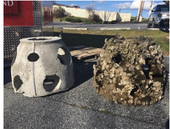
New reef ball (L) and reef ball after 7 months in the water (R). Photo: CCA Maryland
